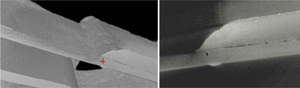
**Fig. 10:** ROI CT of a MIG welding between casting and extruded profile (yellow circle)
