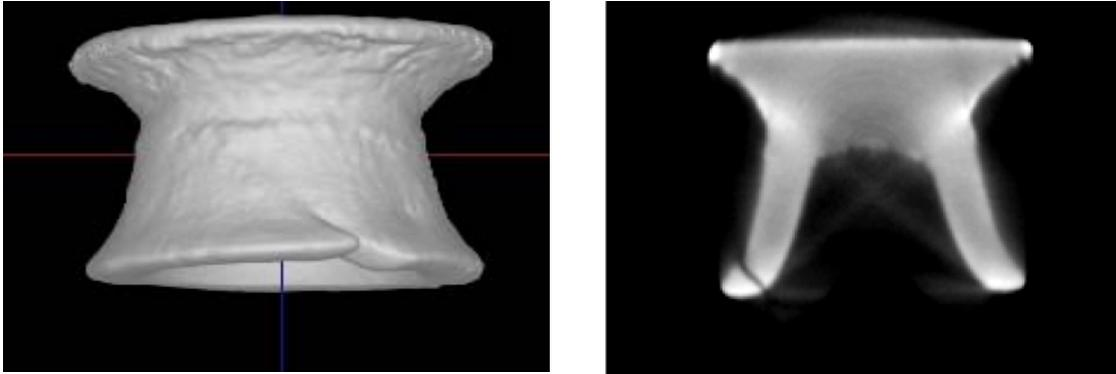
**Fig. 14:** Rivet joint extracted from a car body
