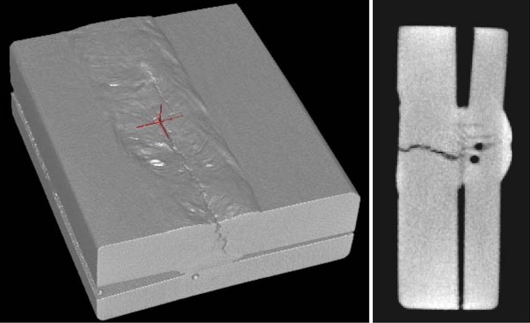
**Fig. 8:** 3D CT of an aluminium laser weld
