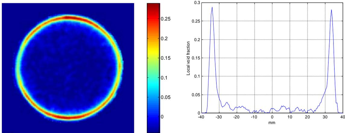
Figure 3: Gas distribution in upward bubbly flow;  $\beta=3.25\%$ ,  $j=1.8$  m/s, elevation 40D.
