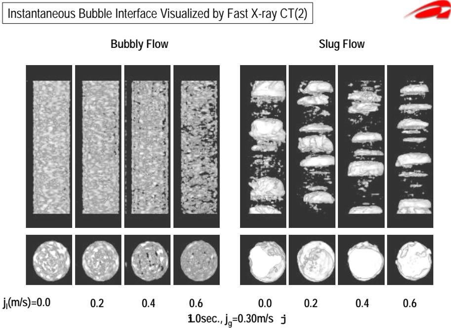
Figure 9: Instantaneous bubble interface visualized by ultra fast X-ray CT for different flow patterns corresponding to four combinations of liquid and gas superficial velocities.
