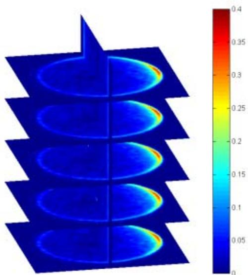
Figure 6: D slices for the gas distribution in Figure 5
