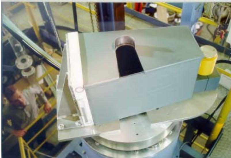
Figure 2: Cone-Beam X-ray tomograph applied to vertical bubbly flow. The pipe (which was removed) is located in the center between x-ray tube (right) and detector (left).
