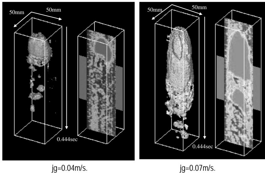
Figure 11: Pseudo-3D representation of gas flow in alumina powder
