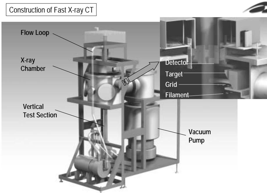
Figure 8: Ultra fast X-ray CT and two-phase flow loop
