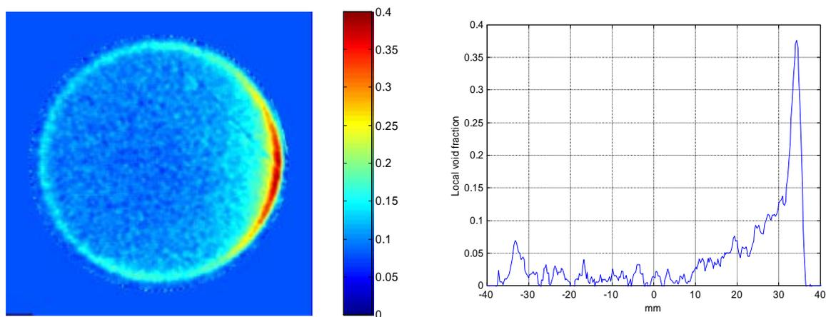
Figure 5: Gas distribution in upward bubbly flow;  $\beta=3.25\%$ ,  $j_l=1.8$  m/s, elevation 40D.
