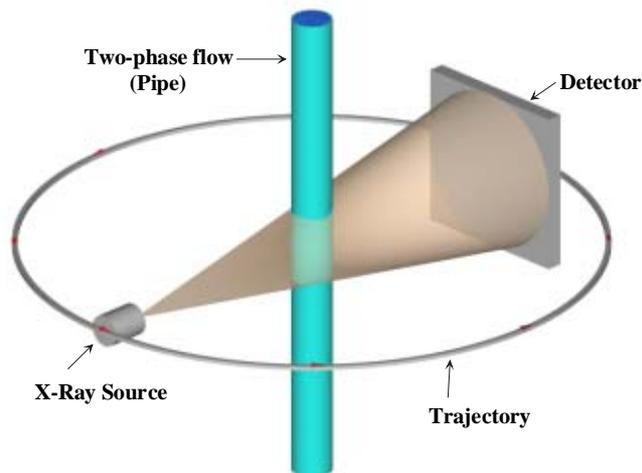
Figure 1: Principle of the cone beam tomography system
