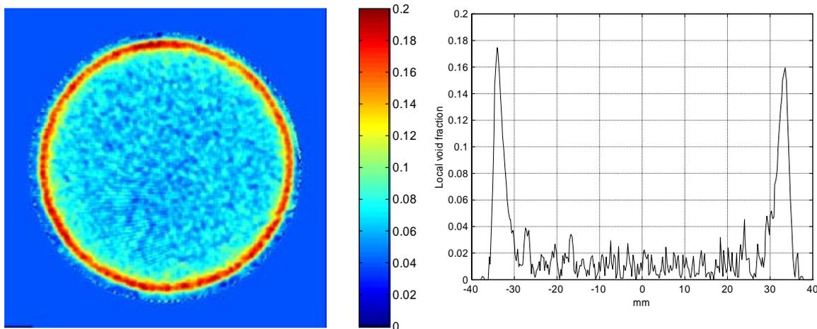
Figure 4: Gas distribution in upward bubbly flow;  $\beta=3.25\%$ ,  $j=1.8$  m/s, elevation 40D.
